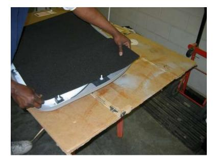
Lay the door panel on a table with the back of the panel facing up. Lay one sheet of Silencer Megabond ¼" foam against the door panel with the white release paper on the foam. Place the edge of the foam just inside the fasteners or clips that secure the panel to the door.
