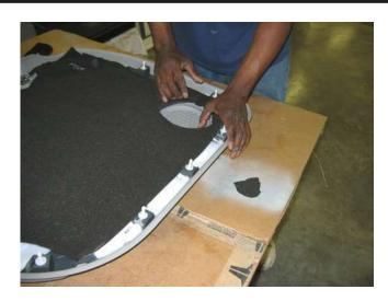
Cut around all panel fastening points, speaker grill, wire harness pass through of any mechanical hardware that will be attached to the vehicle door by slitting the foam and pulling the device through the foam.
