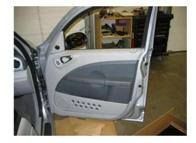
Secure the door panel to the door and the door installation is complete. Repeat the above steps for each door in your vehicle.
