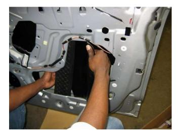
Position the sheet against the outer skin by using the smaller access holes through door frame. Cover a minimum of 60% of the door skin starting in the center and work toward the outer edges of the door.
