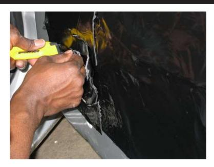
Carefully cut access slits through the HushMat Ultra where wiring or door hardware must pass through. Pull wiring or hardware through slits.
