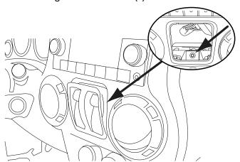
5 Extract (4) 7 mm screws and remove the factory radio.
