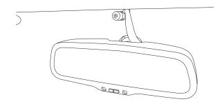
6 Mount the i207-WRA head unit using the factory 7mm screws and return factory panels to their corresponding place
