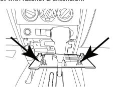
2 Release 2 clips on the top of the bottom panel. This will expose two 7mm screws. Remove those.
