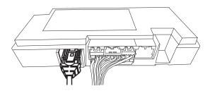
4 Use the USB extension to connect USB adaptor to the radio USB input.
