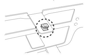
3 Attach the side brackets using the provided 8mm round head screws.
