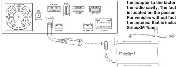
For vehicles with factory SiriusXM connect the adapter to the factory SiriusXM antenna in the radio cavity. The factory SiriusXM antenna is located on the passenger side B-pillar. For vehicles without factory SiriusXM use the antenna that is included with the SXV300 SiriusXM Tuner
