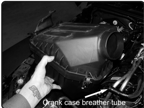
5. Disconnect the crank case breather tube. Then firmly lift up and pull the factory air box assembly out of the engine bay.
