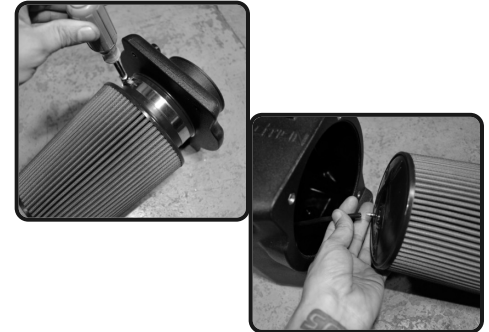
8. Place the filter onto the air box plenum and secure the filter to the plenum. Connect the vacuum line from the Filterminder in figure 6 to the barbed fitting on top of the filter.
