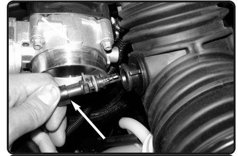
4. Locate the intake air temp sensor underneath the factory air duct from figure 7. Disconnect the harness and twist the IAT sensor to remove the sensor from the air duct.
