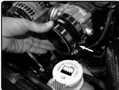
6. Place the 3.25"-3.50" step hose and one #48 and #56 clamp onto the throttle body.
