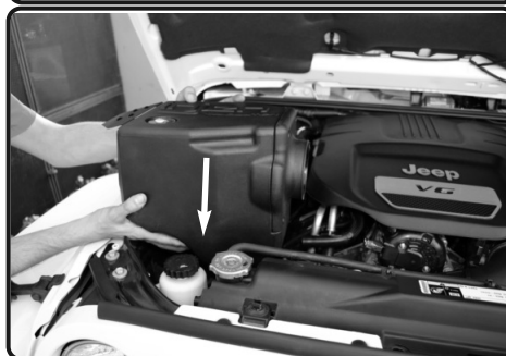
11. Place the Injen air box assembly into the engine bay and line up the pegs below the Injen air box to the factory air box mounting grommets.
