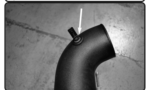
12. Place the grommet onto the 7/8" hole on the injen intake pipe and then insert the intake air temp sensor into the grommet
