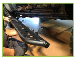
3) Identify the correct Side Step for its corresponding side. The front-end of a Side Step can be distinguished by the first attachment point. The first attachment point will have a taller bracket welded to the Side Step tubing.
