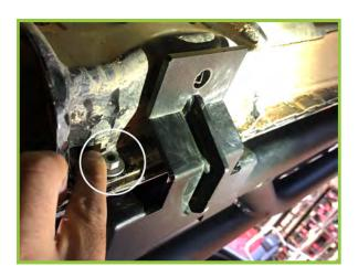
5) Ensure that each stud from the ZROADZ Side Steps extrudes across the body pinch seam. Without tightening at this time, use the 10 Mm Flange Nuts for each pair of horizontal bolts at each attachment point.
