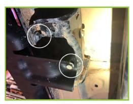
1) Skip to Step 3 if your vehicle is not equipped with the factory Rock Rails. If they are equipped, remove them by carefully untightening the single bolt and the (2) nuts at each attachment point.
