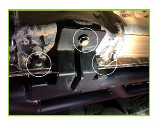
6) Using the provided 8 Mm and 10 Mm bolts, install them into the hole found vertically as shown above. Remember that only the front attachment uses the 10 Mm bolt while the others use an 8 Mm bolt. Once each attachment point has been aligned, tighten each nut and bolt securely. This completes the installation procedure for Z745401 / Z745421.
