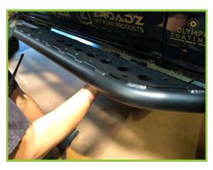
4) Using the same points of attachment from the factory Rock Rails align the ZROADZ Side Steps similarly. If your vehicle did not have factory Rock Rails, locate pairs of 6.5 Mm holes at about 5" apart on the body pinch seam.
