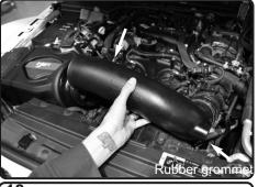
**18.** Install the provided rubber grommmet to the intake tube hole. Insert the Injen intake tube into the vehicle. Position tube to the filter and turbo inlet. Postion for best fit.
