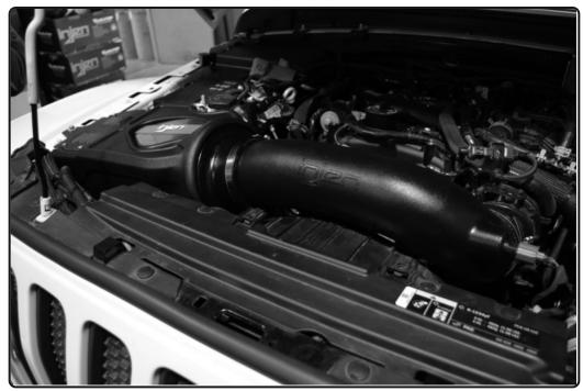
Congratulations! You have just completed the installation of this intake system. Periodically, check the alignment of the intake, normal wear and tear can cause nuts and bolts to come loose. <u>Note: Check clearance and adjust if needed! Failure to check the alignment and adjust the intake can cause damage that will void the warranty. Injen Technology is not responsible for any damages caused by/from improper installation.</u>
