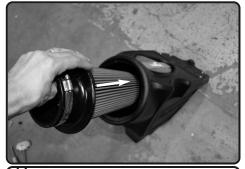
11. Install the twist lock filter into the airbox and secure.
