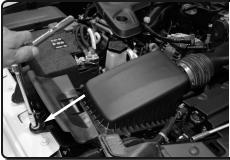
**4.** On the air box, loosen the bolt holding in the airbox. Loosen bolt and save for later install along with the grommet and crush washer.
