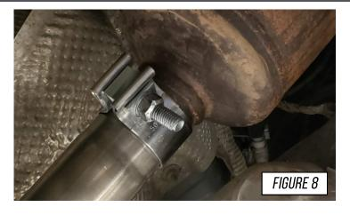
Align the AWE loop pipe flange with the OE flange. It is very important that the AWE pipe and the OE pipe are straight on with each other, as shown in **Figure 9**.
