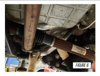
It is crucial to install each section and exhaust band clamps correctly to prevent loose joints, exhaust leaks and rattles.
