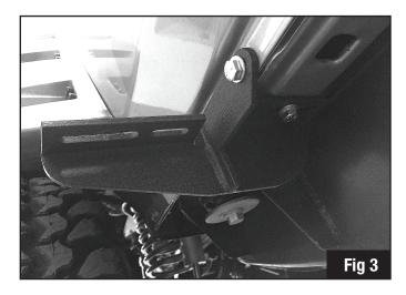
4) Tighten brackets to the body at this time to 18 ft/lbs.
