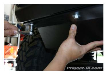
33. Secure the LoD Signature Series skid plate to the lower cross member of your Jeep JK Wrangler using the bolts and washers provided. You will need a 9/16" socket and wrench for this job.
