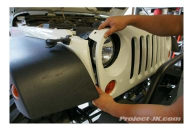
**25.** Lean your Jeep JK Wrangler's grille forward a bit to gain access to the indicator lights. Then, take the wiring harness plug and pull the red locking tab back.
