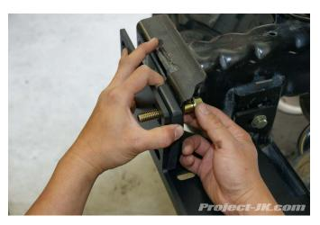
15. Repeat step #14 until all the steel spacers are installed in between the LoD Signature Series winch plate and frame rail bumper mount and that all the bolts are sticking through them as shown in this pic.
