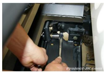
**18.** Accessing the bolts and nuts through the fog light holes on your LoD Signature Series JK Front Winch Bumper, tighten up the (4) mounting bolts and nuts located on the outside of your Jeep JK Wrangler's frame rails using a 3/4" socket and wrench.
