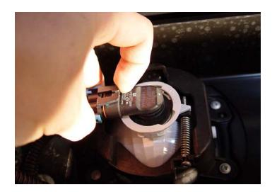
**5.** Using a pair of needle nose pliers, pry off all the fog light wiring harness connectors on the back of your Jeep JK Wrangler's front bumper.
