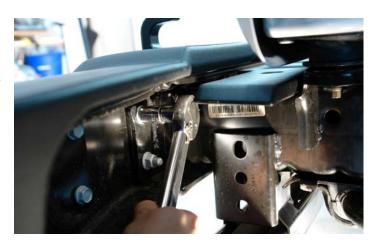
**8.** Remove the backing plates off the bumper mounting studs as shown in this photo.
