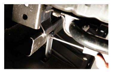
**4.** If your Jeep JK Wrangler came equipped with factory fog lights, climb under the front of your Jeep, look up behind the front bumper, locate the wiring harness plug, lift up the clip and then pull it off as shown in this photo.
