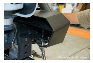
**19.** Using a 3/4" socket, tighten up the LoD Signature Series winch plate frame rail mounts as shown in this pic.
