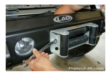
**29.** Carefully place your winch on top of the LoD Signature Series winch plate and then reinstall your Jeep JK Wrangler's grille as shown in this pic.
