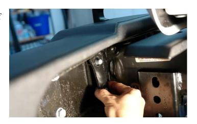
**9.** Carefully pull off your Jeep JK Wrangler's front bumper off the frame rails. If your JK came equipped with factory tow hooks, grab and use both of them to carefully pull your front bumper off the frame rails.
