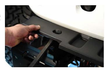
12. Again, if your Jeep JK Wrangler came equipped with factory fog lights, use a phillips screwdriver to remove the 4 screws securing them to the bumper. Then, pull the fog lights out and set them aside until you are ready to install them in your new LoD Signature Series JK Front Winch Bumper.
