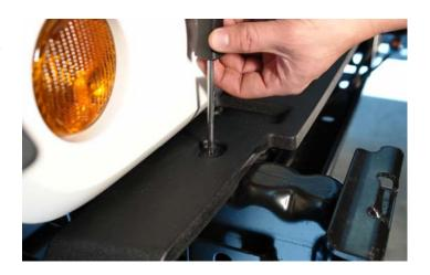
**11.** Again, if you find these screws to just spin in place, use a flathead screwdriver or small pry bar to help you lift up the cover off the frame rail and force the screw out.
