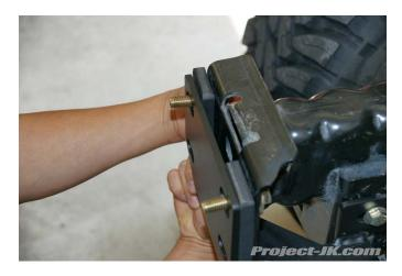
16. With the help of a friend, carefully place your new LoD Signature Series JK Front Winch Bumper on to the frame rails of your Jeep JK Wrangler and slide the mounting holes through the bolts you just installed. Reaching from the back, loosely secure it in place using the nuts provided.
