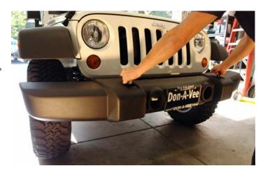
**10.** Using a phillips screwdriver, remove the 2 plastic screws securing the top plastic cover in place.
