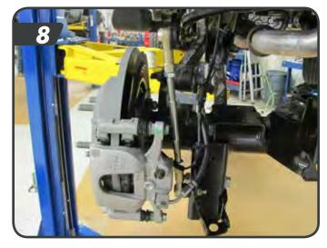
c. Install the rear bump stop spacers on the axle with slant cut facing forward. Fasten the bump stop spacer to the axle with the  $5/16'' \times 7/8''$  bolts, nuts and washers. Torque bolts to 20 ft-lbs. ( $\frac{1}{2}$ ") [4 - 3" extension shown]
