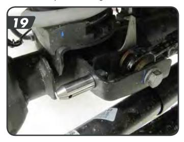
s. Install the longer disconnect post on the driver side axle sway bar link mount with it pointing inboard [20]. Fasten with the ½" nylock nut and tighten to 65 ft-lbs. Tighten the post with the pin hole parallel to the ground. Slide the polyurethane spacer on the pin up against the axle tab.
