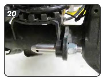
t. The kit comes with disconnect retention brackets to hold the links when the links are disconnected. Install the retention brackets using the provided 5/16" bolts into the factory hole in the front of the coil bucket [21]. These are designed to slightly interfere with the edge of the coil bucket to hold them in place.
