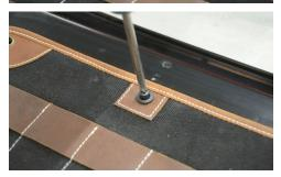
Tighten the each screw snugly, being careful not to over-tighten
