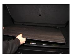
**STEP 2**Fold the rear seat forward, and remove the floor panel.
