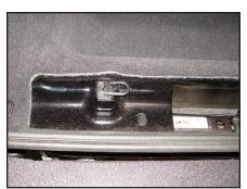
Position the floor panel clip as pictured to allow it to fit in the void in the bottom of the Stealthbox®.
