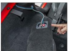
Connect speaker cable to the terminal cup on the Stealthbox®, and place the enclosure into position between the Front and Rear Brackets. Route the speaker cable as necessary.
