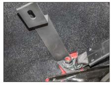
Slide the Front Bracket over the factory stud, followed by the seat belt bracket and nut, as shown. Hand tighten.
