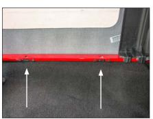
Locate the two indicated holes at the top of the side rail.
