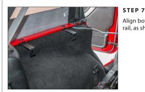
Align both Rear Brackets perpendicular to the rail, as shown.
