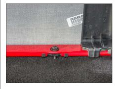
Slide a 3/8 " Flat Washer and a 3/8" Nylon Washer over an M8 x 30 mm 1.25 Flange Head Bolt (substitute an M8 x 45 mm 1.25 Flange Head Bolt for vehicles with hard top), and thread the assembly through one of the holes indicated in the previous step. Repeat for the second hole.
