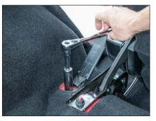
**STEP 2**Fold the rear seat down, remove the nut at the base of the seat belt bracket, and slide the bracket off of the stud.
