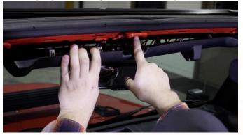
With a T25 Torx bit, unscrew and remove the footman loop, save factory bolts for future use if needed.
