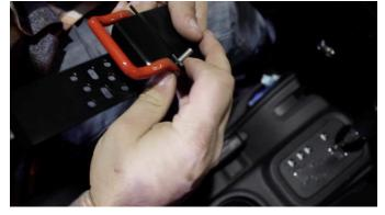
Insert the included bolts through the front and begin securing the mount and footman loop back into the windshield frame, using a Philips screwdriver.
