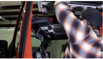
Gently and evenly pull down on the cover to release the body clips, revealing the footman loop.
