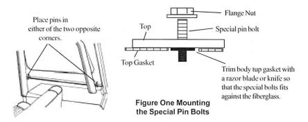
Next, replace the top back onto the Jeep, being careful to set the newly installed pins through the appropriate holes in the Jeep body tub. Then, assemble the clamps as shown and install as in figure 2. Tighten the black knobs securely. Check for tightness again after 25 miles. For additional protection for your paint on the body tub rail, we recommend our Paint Saver. See *your dealer* for more information.
