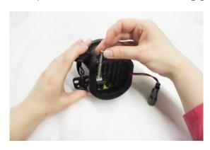
7. Plug in the lamp and turn on the fog lamps while holding the lamp in place. Compare the pattern of the light coming from the 2 fog lamps as the shine on the wall by covering and uncovering each lamp individually.
