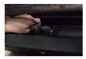
9. When the existing and new fog light horizon lines are aligned, use the 4 existing mounting screws to install the lamp assembly to the bumper.
