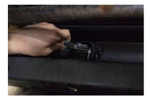
2. Remove the 4 Phillips screws from existing fog lamp with a Phillips screwdriver and save the screws. Remove the fog lamp from the vehicle.
