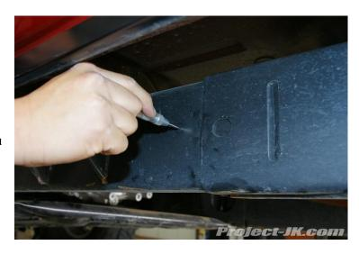
**11.** Using a small metal drilling bit or Unibit, begin drilling pilot holes on all the mounting points on you've marked off your Jeep JK Wrangler's frame rail.
