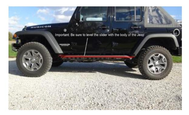
**Important:** Before marking or drilling any holes be sure to make sure that the slider is positioned properly. The slider needs to be aligned so that it maintains an even spacing between it and the pinch seam of the body.
