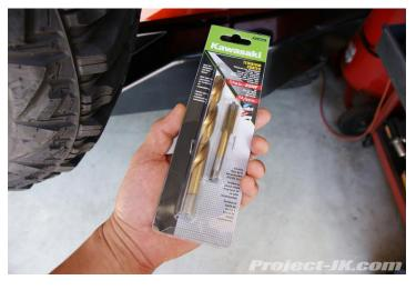
**13.** Using the drill bit that comes with the drill and tap set, finish drilling out all the pilot holes that you made back on step #11.
