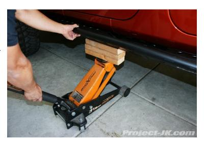
17. Using the factory hardware, secure your new LoD Signature Series Rock Slider to the points where the automatic transmisson and transfer case skid plates attach the frame rail on your Jeep JK Wrangler. An 18mm socket will be needed for this job.
