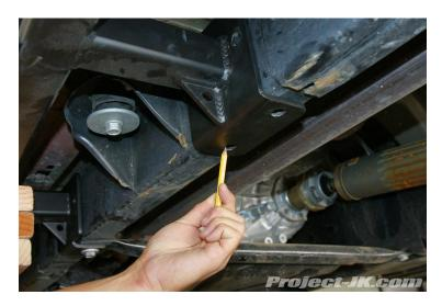
**9.** Remove the 2 bolts securing your LoD Signature Series Rock Slider onto the frame rail and then carefully lower and remove it from your Jeep JK Wrangler.
