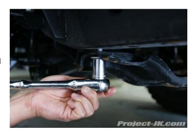
**5.** Maneuver your LoD rock sliders into place underneath the jeep. The rear mount of the sliders has 4 bolt holes so the sliders will need oriented so that the mounts with 4 holes are to the back of the Jeep.
