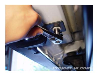
**3.** With the 6 nuts and 3 bolts removed, the factory rocker guards or running boards on your Jeep JK Wrangler Unlimited Rubicon or Sahara should pull off the body pinch seam with ease. Set them aside.
