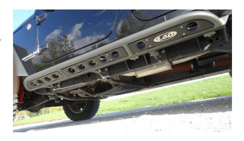
20. With both sliders installed on the Jeep install the lower side panels. Use the ½" x 5/8" button head bolts provided. The logo should be place to the rear of each slider as shown in the picture to the right.
