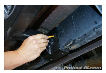
**8.** On the mount closest to the rear tire, there are 2 holes on the bottom of your Jeep JK Wrangler's frame rail that you will need to mark off as well.
