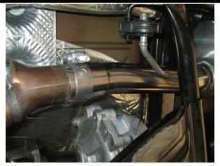
**Step 1.** To remove the OEM exhaust system, unbolt the clamps at the catalytic converter and over-axle pipe. Disengage the welded hangers from the rubber isolators and remove the components. You may need to temporarily remove the transmission skidplate to aid in removal and installation.
