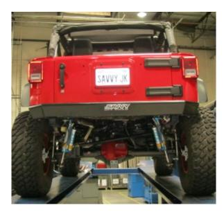
**Step 4.** Once a final position has been chosen for the new exhaust system, evenly tighten all clamps from front to rear using the torque specifications on page one of the instructions. Inspect all fasteners after 25-50 miles of operation and re-tighten if necessary.
