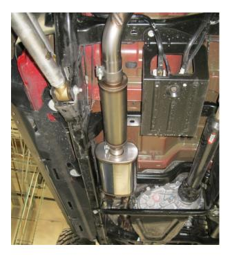
**Step 2.** Being installation of your new system by fitting the Muffler Assembly inlet pipe to the catalytic converter outlet. Locate the welded hanger to the rubber isolator. Secure using the supplied clamp. Be sure to fit the OEM alignment peg in the larger notch. Leave all clamps loose for final adjustment.
