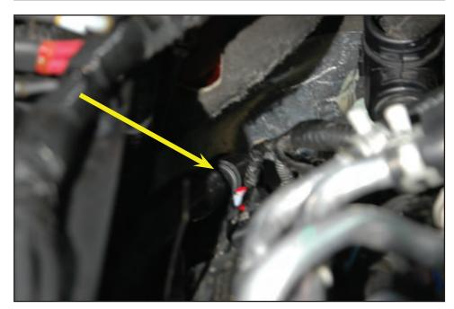
120. Connect the other 45° connector end to the right hand side PCV hose barb on the supercharger inlet shown with a yellow arrow. Tighten the heater hardlines at the two stud locations. Install the provided swivel spacer, and two 1/2" x 15" cable ties in the location shown with a red arrow.
