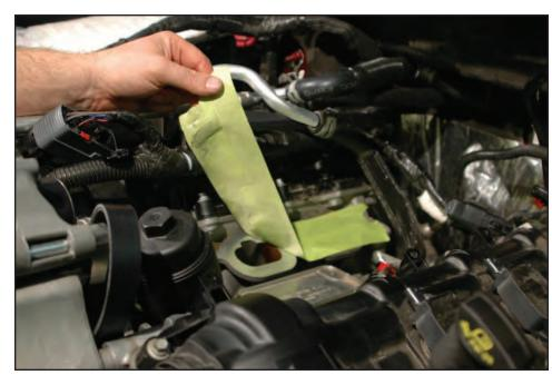
105. Use isopropyl alcohol or some other non-petroleum based solvent to wipe the head surfaces clean of any tape residue.
