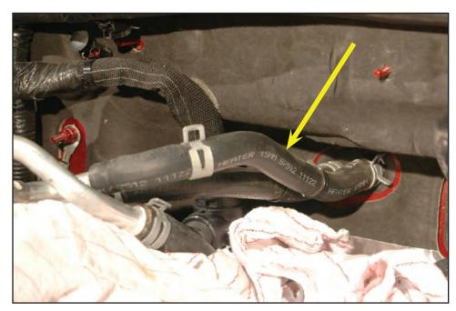
102. Use two provided 4" x 18" x 5/8" 90 ° elbow hoses and the provided 5/8" x 5/8" 90 plastic elbow (coupling) to create this replacement heater hose assembly. Cover the long straight leg with the provided split loom as shown. Secure coupling (hose-mender) with provided 5/8" spring clamps. Verify the dimensions using your vehicle hard line heater barbs. This image also displays the orientation, with the top of the picture being the firewall end of the assembly.
