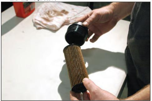
14. This shows the provided new two piece filter element orientation.
