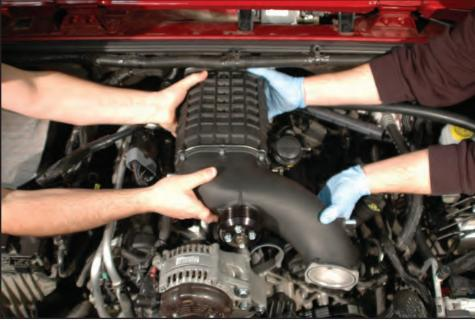
107. Use a telescoping magnet tip to set the supercharger mounting bolts in position. The four long bolts go in the front and rear mounting holes, and the short bolts fill the center mounting locations.
