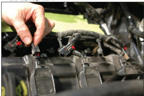
65. Carefully pull out the four (two each side) wire loom mounting tree connectors holding the injector/coil wire looms to the valve covers.
