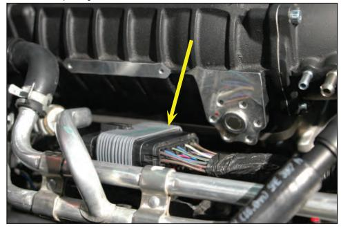
122. Inspect the O-ring installed in the throttle body flange for damage, if damaged call Magnuson for a replacement. Install the OEM throttle body on the new supercharger inlet using the four provided bolts. Torque the bolts to 106 in-lbs. Verify your torque wrench settings.
