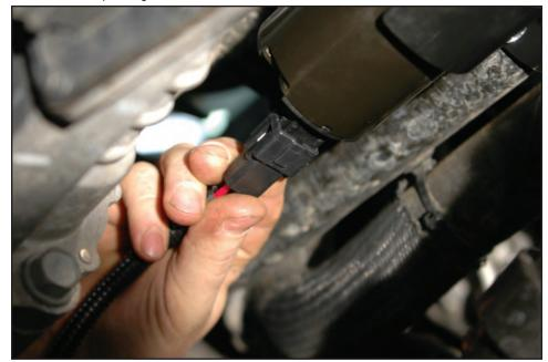
152. Connect the provided EVAP tube connection to the vacated barb near the inside end of the fuse center.
