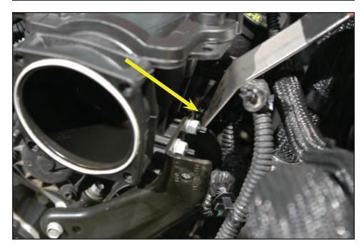
36. Use a 10mm wrench to remove the four upper intake manifold mounting bracket fasteners from the left hand side of the engine. Two are at the forward bracket and two at the rear bracket.
