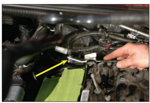
69. Use a shop vacuum to clean any debris from the intake ports of the heads.
