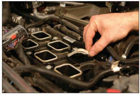
53. Use a shop vacuum to remove any debris on and around the intake manifold.
