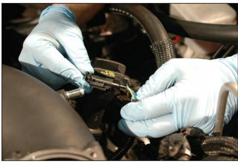
112. Connect the provided MAP sensor extension onto the MAP sensor connector behind the supercharger, just below the charge air cooler hose connections on the intake manifold.
