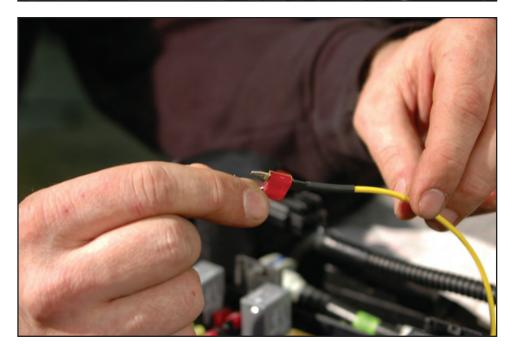
150. Reinstall the fuse in the fuse center M37 slot incorporating the fuse tap.
