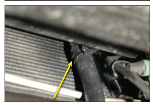
141. Cut the long leg of the 4" x 40" x 3/4" 90° elbow hose to fit and connect to the forward hose barb on the reservoir using a worm gear clamp. It's important to utilize only worm gear clamps on the reservoir. For clarification see the plumbing diagram at the back of this instruction manual.
