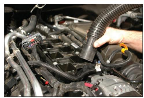
54. Use isopropyl alcohol or other non-petroleum based solvent to carefully wipe clean the intake manifold ports.
