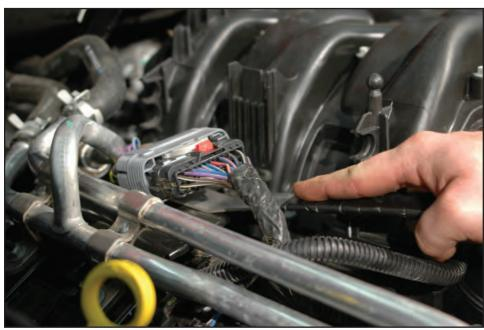
43. Use a 10mm socket to remove the fasteners holding the right hand side heater tube/wiring harness bracket to the engine. Two bolts are closest to the intake manifold, two nuts are holding the heater tubes to the bracket, and two other nuts are near the base of the valve cover, between the battery-box and where the bracket bends down toward the exhaust manifold. (see next step)
