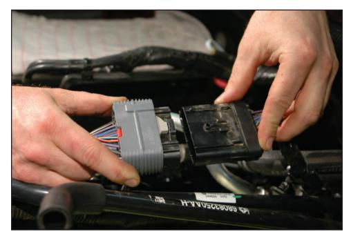
99. Route the rear harness under the existing heater hose connecting to the hard line coming up from the back of the engine compartment. It does not need to be reconnected at this time.
