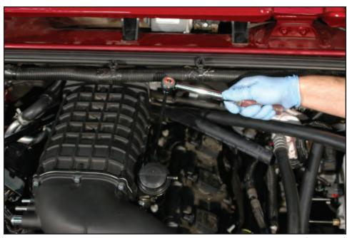
109. Use this image to sequence the torquing of your mounting bolts. Do NOT torque each bolt down to full specs in a single step. Rather, gradually bring each bolt up to spec rotating in this pattern.
