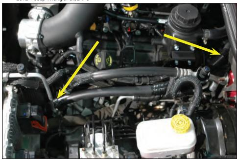
134. Cut the hose as necessary to fit and connect to the upper LTR hose barb using a provided spring clamp.
