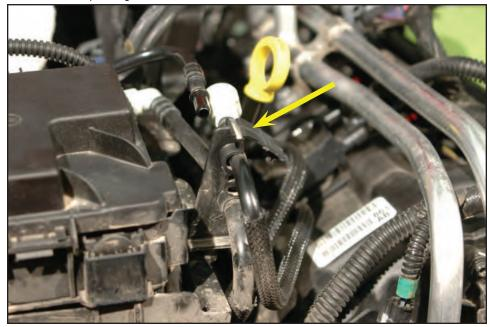
59. Remove the forward section of the EVAP tube from the vehicle.
