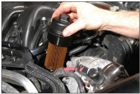
13. Pull the cap off the OEM filter element.
