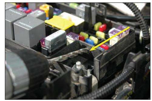
147. Use a 13mm wrench to remove the nut from the hot terminal of the fuse center and replace incorporating the ring terminal on the red wire from the intercooler pump wiring harness.
