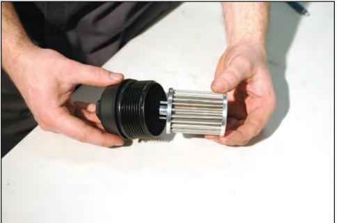
17. Replace the oil filter casing cap onto the filter housing and torque to 18 ft-lbs using a 24mm socket.
