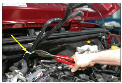
96. At the firewall, pull the four center-most cross vehicle wire loom mounting tabs off of the mounting posts. Use the center most mounting clips to "hold" the harness up using the hood rear seal. Alternately, you can tie the loom to the hood-deck support brackets using provided zip-ties.
