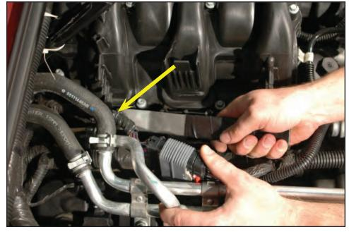
50. Use an 8mm socket to remove the seven intake manifold mounting fasteners. Three are on the top, and four are at the base of the intake manifold. Pull up and twist the upper mounting bolts counter-clockwise to have the bolts held in the extended position.
