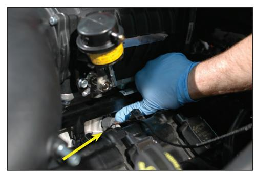
111. Connect the free end of the IAT extension harness to the existing IAT plug near the throttle body flange of the supercharger.
