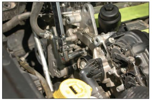
83. Install the provided drive belt following the diagram at the back of this manual. At the top, create the triple-loop configuration shown. Use a zip tie to loosely hold the belt.
