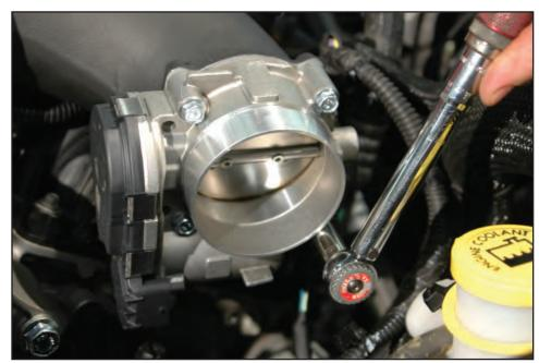
123. Reconnect the throttle body control harness to the throttle body and press the harness mounting clip back on the throttle body mounting tab/boss.
