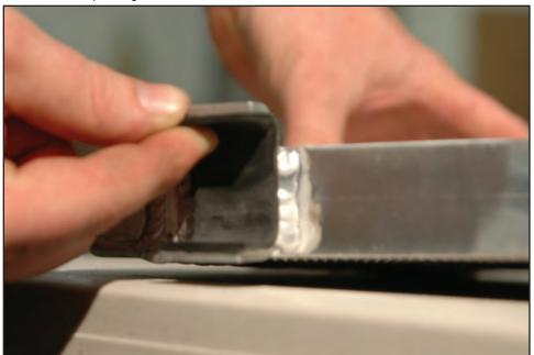
131. Press the LTR mounting brackets on the lower cross frame rail, and roughly align the holes with the existing holes in the upper cross frame brace. Slide the provided double nut plate up and into the channel of the upper cross frame brace, and align the nuts with the two existing holes located behind the wiring harness.
