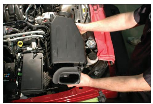
30. Disconnect the harness clip from the tab/boss on the throttle body. Pull out on the red throttle body control locking pin, and then press down on the exposed end to release the plug from the throttle body.
