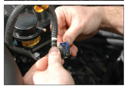
117. Snap the fuel line back onto the fuel rail at the front barb of the left hand side fuel rail. Press the locking clips back into secure position. Pull on the fuel line. It should not be able to be removed without releasing the locking clips.
