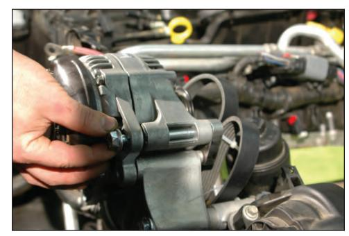
90. Torque the M10 fasteners with a 15mm socket to 40 ft-lbs. Torque the M8 fasteners with a 13mm socket to 25 ft-lbs. Verify your torque wrench settings.
