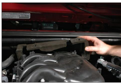
21. Disconnect the windshield washer tube from its connector on the left side of the firewall
