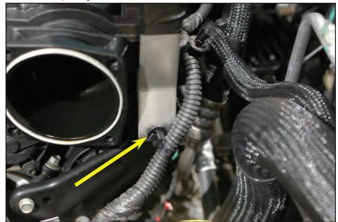
35. Remove the harness mounting "tree" clip from the back of the upper intake manifold mounting bracket.
