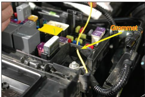
149. Install the provided fuse tap at the end of the yellow wire on one leg of the M37 fuse (fuel pump relay removed earlier).
