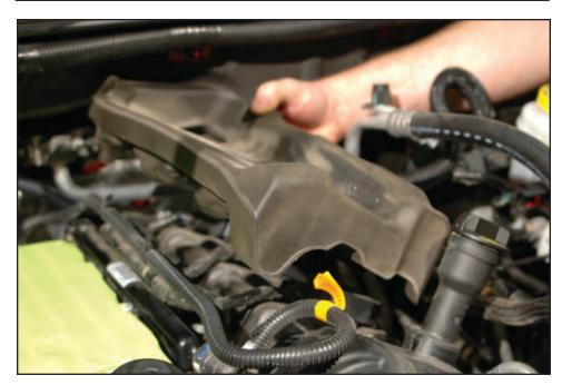
57. Disconnect the EVAP hose by the fuse center by pulling up on the release tab and separating the two components. These are located next to the fuse box.
