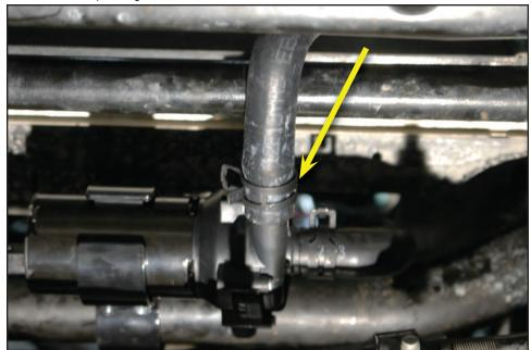
140. Cut the remaining section of the 4" x 18" x 3/4" 90° elbow hose to fit and connect to the lower hose barb on the LTR using a provided spring clamp.
