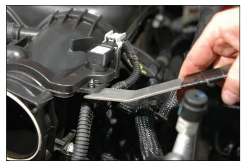
33. Disconnect the Manifold Absolute Pressure (MAP) sensor from the left side upper intake manifold, near the throttle body mounting location by pressing the release tab and pulling free.
