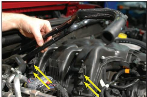
41. Remove the PCV vacuum tubes connected to the back of the valve covers from the vehicle. The left hand side PCV tube will be reused and components of the right hand side PCV tube will be reused. If it's difficult at this time to remove the tubes completely, it's helpful to tuck the tubes up out of the way by securing to the cross deck wiring harness using the provided zip ties.
