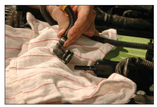
63. Pull up on the fuel injector locking clips, and squeeze the release tab to remove the six fuel injector connections (three each side).
