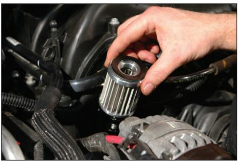
16. The upper filter element with the extrusion gets pressed into the oil filter casing cap with the extrusion going into the cap. This will "snap" into place holding the element to the cap.
