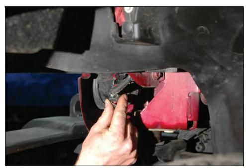
162. Cut 1-1/2" off the end of the PCV hose on the right hand side of the engine and reconnect to the air box hose barb.
