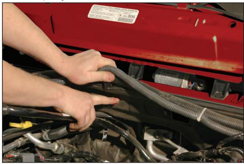
98. On the right hand side the main wiring harness runs parallel to the valve cover. At the center connector, first pull the red locking clip out, then slide the gray sleeve over (to the left in this picture) to allow this connection to be separated. Disconnect the plug.
