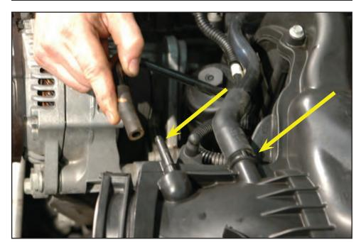
39. Pull the brake booster vacuum hose from the front-left side of the upper intake manifold.
