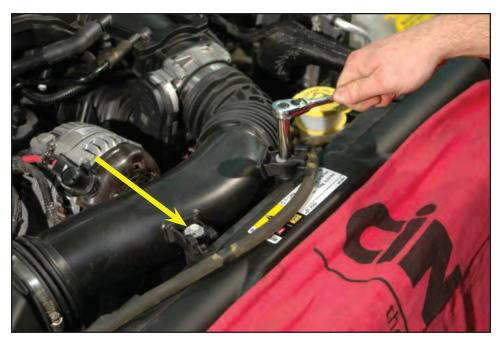
24. Use an 8mm socket to loosen the throttle body mounting clamp at the air tube to throttle body connection.
