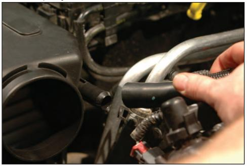
29. Pull up on the air box to remove the assembly from the vehicle. Set aside for later reinstall.
