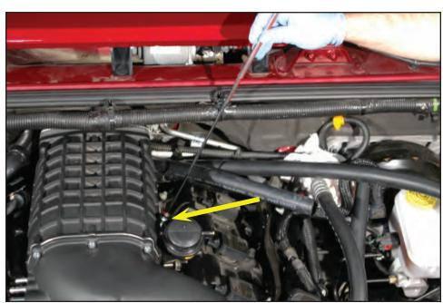
108. Torque all mounting bolts to 106 in-lbs. Use the multi-step tightening sequence shown in the next image.
