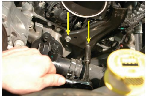
38. Pull the EVAP hose and the PCV hose off the hose barbs on the front-right side of the upper intake manifold.
