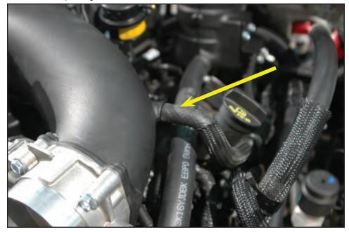
155. Align the three pins on the bottom of the air box with the three grommets on the air box tray and press the air box back in original position. This will "snap" in place.
