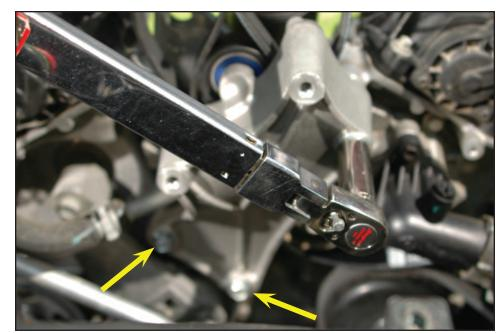
87. Press the offset alternator nut into the upper mounting hole of the alternator mounting bracket as shown.
