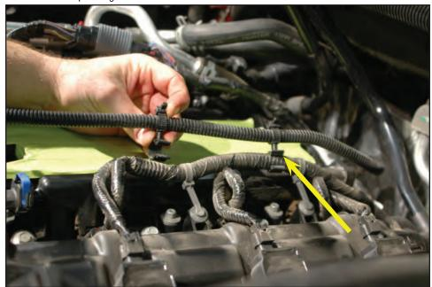
62. Rotate the fuel line to expose the white locking clip on the bottom. Carefully remove this locking clip out and pull the fuel line off the fuel rail. Have some shop rags handy to catch any residual fuel in the fuel line. Dispose of contaminated shop towels in an appropriate manner.
