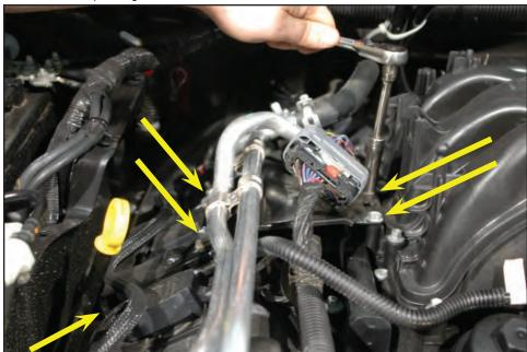
44. This picture shows the engine out of a vehicle for clarity and illustrates the location of the two lowest bracket mounting nuts.
