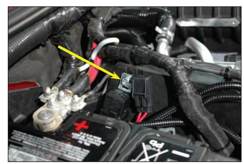
144. Route the split loom covered power connector with the yellow wire incorporated forward. Utilize the vacated clamp of the EVAP center as a mounting point and secure the harness in position by pressing the hinge clamp down over the split loom.
