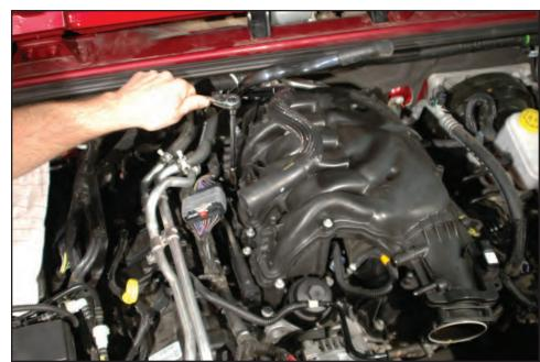
51. Lift up on the right hand side of the upper intake manifold then slide the assembly to the right while lifting to remove the assembly from the vehicle.
