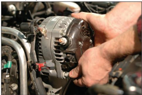
89. Tighten the M8 x 100mm fastener in the left hand side mounting location engaging the previously installed offset alternator nut.
