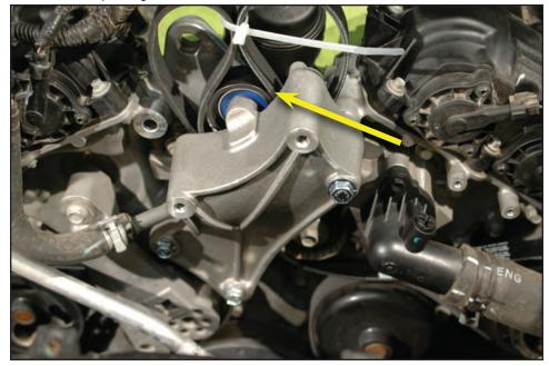
86. Torque the mounting fasteners to 25 ft-lbs for the 12&13mm headed bolts, and 40 ft-lbs for the 15mm headed mounting bolt. Verify your torque wrench settings.
