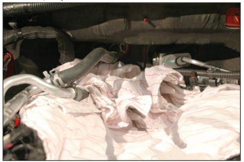
101. Before removing the heater hose, loosen the radiator cap to relieve any pressure still in the system. Disconnect the center most heater hose running from the firewall forward, and angling over toward the right hand side fender to connect to the hard line. There will be some fluid in the hose and barbs, the shop towels should take care of this residual fluid. Dispose of contaminated towels appropriately.
