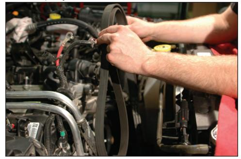
80. Use a 13mm socket to remove the right idler pulley that is just above the tensioner pulley.
