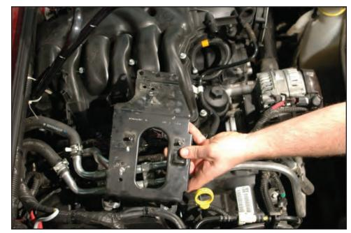
48. Place the provided mounting bracket down toward exhaust manifold and slide it up and under the heater lines. Reconnect the bracket to the studs near the base of the valve cover and secure with a 10mm socket. DO NOT reconnect the heater hard-lines to the studs on the new mounting bracket with the OEM nuts at this time. Reconnect the two tree connectors to the holes on the new bracket. Install the provided 1/2"OD x 1/4"ID x 3/16" spacers over the studs shown with red arrows.
