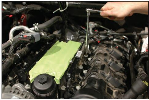
68. Pull the lower intake manifold forward and up. There is one remaining wire loom tree connector that needs to be carefully pried out of the rear of the intake manifold prior to pulling the manifold out of the vehicle. Remove this connector and set the lower intake manifold aside. There will still be residual fuel in the fuel rails, so cap this line and have rags or shop towels ready to catch any spilled fuel. Dispose of contaminated shop towels in an appropriate manner.
