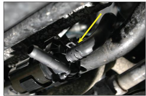
139. Connect the short leg of the 4" x 18" x 3/4" 90° elbow hose to the discharge barb of the intercooler pump using a provided spring clamp. Angle the remaining hose toward the left hand side a bit to point directly at the lower LTR hose barb. This hose will be running below the sway bar.
