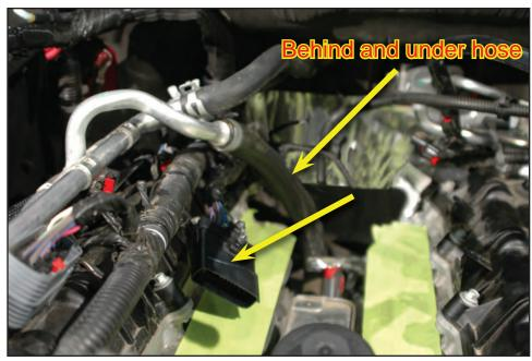
100. A heater hose needs to be removed. There will be some residual coolant in the hose, to protect the ports, place some shop towels down over the intake ports of the heads in the valley cover. The tape should still be covering the ports at this time.
