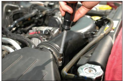
26. Disconnect the IAT electrical connection leaving the OEM IAT sensor in place.
