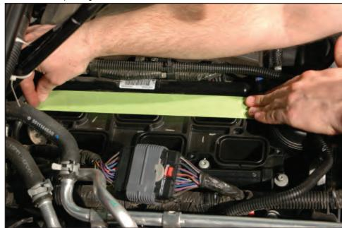
56. Remove the left hand side foam insulation from over the valve cover.
