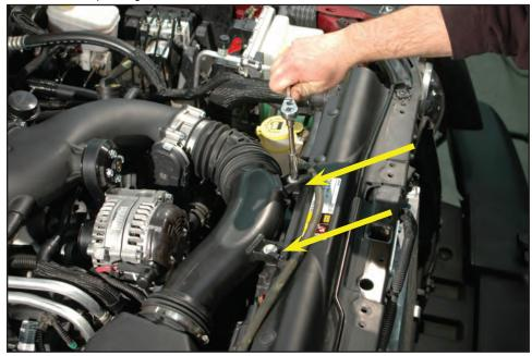
158. Press the overflow hose back on the two clamps by the mounting bolts of the air tube.
