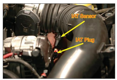
27. Carefully pull the air tube off the throttle body and air box. Set aside for later reinstall.
