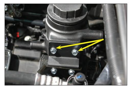
126. Cut to fit and connect the right hand side charge air cooler hose (2.5" x 18" x ¾" 90° angle hose) straight end to the upper hose barb on the intercooler reservoir. Caution: only use the provided worm gear clamps on the reservoir bottle.
