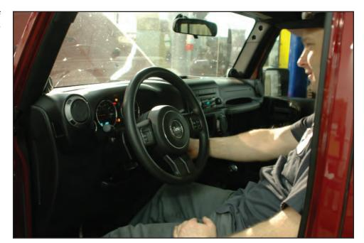
9. Remove the negative battery terminal using a 10mm wrench. Slide the battery cable out of the way and apply some insulation material like tape to it so that it cannot make accidental contact with the battery terminal.
