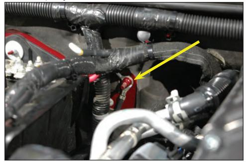
146. Remove the fuse box cover. Use a 1/4" drill bit to drill a small hole in the back wall of the fuse center power lead. Center the hole between the existing fuses beyond as shown.
