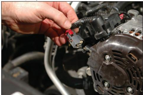
74. Disconnect the alternator positive battery cable using a 13mm socket.
