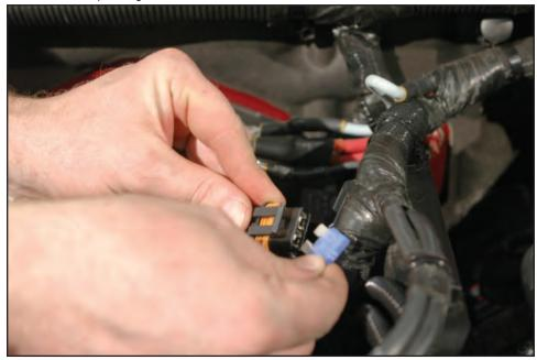
143. On the inside surface of the battery tray toward the rear there are two holes. Using the provided hardware, attach both the fuse center and the relay to the front hole as shown in this picture.
