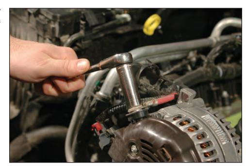
75. Remove the two upper 15mm alternator mounting bolts securing the alternator to the engine and the two lower 13mm bolts holding the alternator to the mounting bracket.
