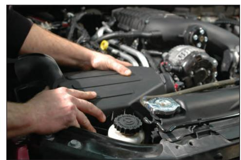
156. Connect the OEM air box to the throttle body and air box and secure with the OEM clamps.
