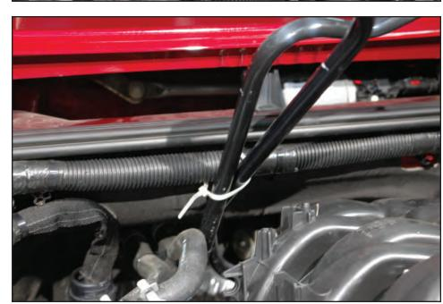
42. Using the tree clip removal tool carefully pry up on the base of the right hand side main wiring harness connector to release the two mounting tree clips from the bracket below.
