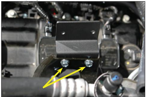
125. Use a 10mm socket and provided fasteners to mount the reservoir to the two mounting holes left on the reservoir mounting bracket just installed. Torque all four fasteners to 106 in-lbs.
