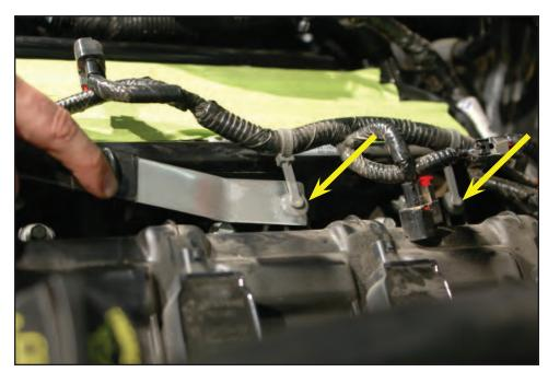
66. Tuck the left hand side wire loom out of the way to the left hand side of the engine compartment.
