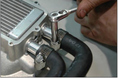
94. Remove the OEM gaskets from the OEM intake manifold, clean and inspect for damage, if damaged replace with OEM gaskets from your Jeep dealer. Install in the grooves on the bottom of the supercharger intake manifold. Do not allow any debris to fall into the supercharger intake manifold.
