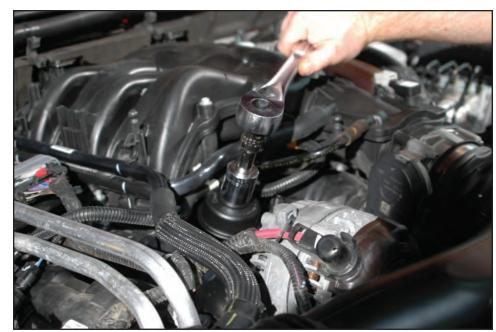
12. After a couple of minutes, pull up on the casing and remove the existing filter element which will be snapped into the cap.
