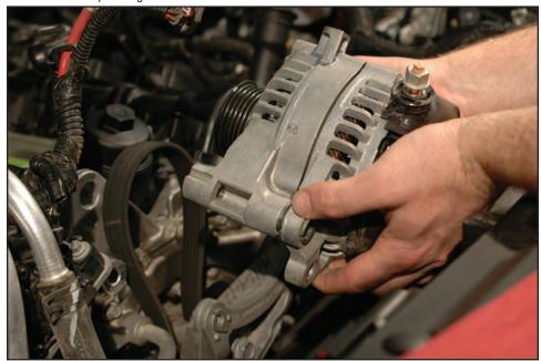
77. Remove the two remaining fasteners holding the alternator mounting bracket to the engine using a 13mm and 16mm socket.
