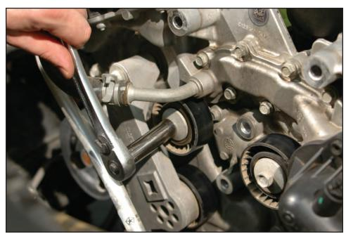
81. Install the provided low profile fastener in the vacated hole adjacent to the remaining idler pulley above and to the left hand side of the tensioner pulley. Note: For clearance reasons this bolt does not have a washer
