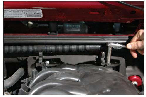
20. Pull the insulation away from the manifold.
