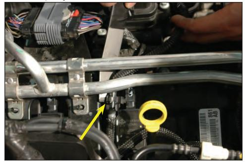
47. Lift up on the heater lines, slide the bracket down toward the exhaust manifold and remove the bracket from the vehicle. This bracket will not be reused, store it in a safe place if you intend to return the vehicle to stock at a later date.
