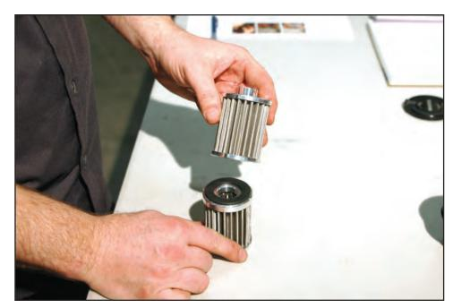
15. Place a thin film of new oil on the lower filter element gasket and slide into the oil filter casing on the engine with the gasket pointing up.
