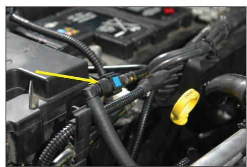
153. Connect the free end of the hose to the center barb on the supercharger on the right hand side of the inlet.
