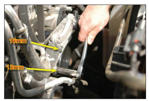
78. Remove the alternator mounting bracket. This bracket will be replaced with a provided bracket. Set aside in case you ever want to return the vehicle to factory condition.
