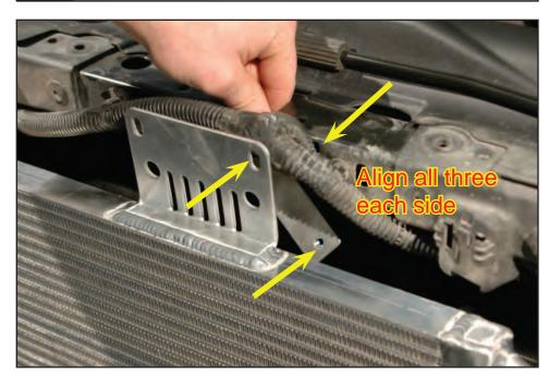
132. Do some final adjusting as necessary and mount the upper LTR mounting bracket to the upper cross frame brace, engaging the two nuts of the double nut plate with the provided bolts. Secure using a 10mm socket.
