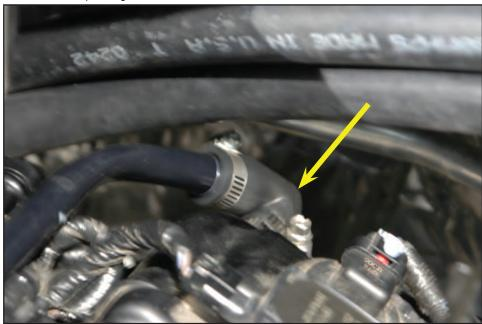
119. Use two provided hose couplings/menders to the ends of the provided 5/8" fuel vapor hose. Remove the OEM PCV hose ends from the removed right hand side PCV tube assembly. Place one end on each hose coupling. Connect the larger connector end to the PCV barb at the rear of the right hand side valve cover.
