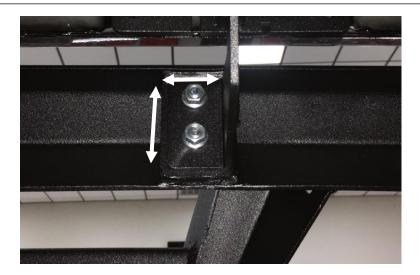
**<u>Step. 8</u>**: After finial positioning, completely tighten all (x6) ¼"-20 x ¾" in the pinch weld attachment. <u>Step. 9</u>: Next, tighten all (x3) upper body mount positions to 17-20 Ft/lbs. torque. <u>Step. 10</u>: Repeat steps 2-9 for passenger side.
