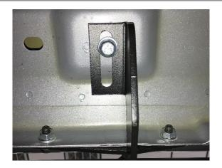
**Step. 6** Next, start all (x6) ¼-20"x 3/4" hex bolts, (x12) M8 flat washers, (x6) 5/16" lock washers and (6) ¼"-20 HC Nut in the pinch weld mounting locations and leave loose for now.
