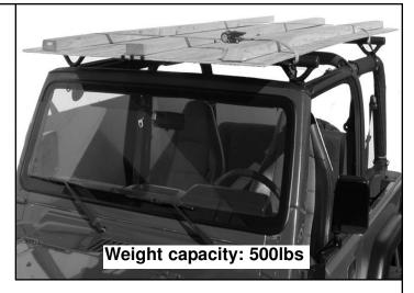
**Tools Needed:** 3/8" drive ratchet wrench; Socket sizes: 1/2". 9/16"; Combination wrench sizes: 1/2", 9/16"
