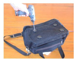
4. Without changing the position of the compressor in the bag, turn the bag and compressor over so the bottom is facing up. Secure the plywood to the bag using the screws supplied with the feet by screwing through the fabric into the plywood.
