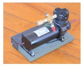
2. Mount your compressor on a 7" x 12" piece of 1/2" or 3/4" plywood. Offset the compressor to one side of the board so it will end up as shown in photo 3 below left.
