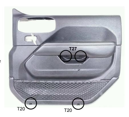
2. Starting at the bottom, pull the panel away from the door. The goal is to pull the lower half of the panel out far enough to release the pins that secure the panel to the door.
