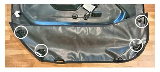
In the photo at right the push pin is misaligned with the hole it pushes into. Ensure that all push pins are properly aligned when pushing the door panel back in place.
