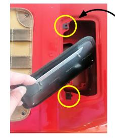
2. Slip the clip-nuts over the holes the clips came out of.
