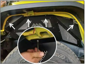
Step 4. Place inner fender back onto vehicle. Line up the holes in the inner fender with the holes on the vehicle and previously drilled holes. Place a M6x16mm Allen head bolt with supplied M6 flat washer through the hole in the inner fender onto the vehicle as shown. Finger tighten only.
