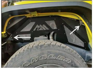
Step 1. While holding the inner fender in place using a white marker mark the area for drilling as shown. Remove inner liner.
