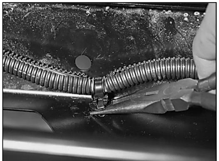
Step 8. Using a fastener pry tool remove the wiring harness connector attached to the back of the bumper.
