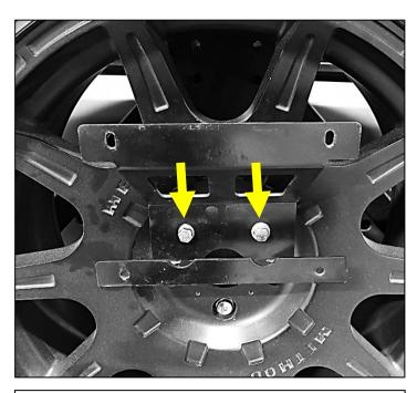
Step 3. While holding the license plate holder in place, place a supplied M8x1.25x20mm hex head bolt with supplied M8 split washer (E) and supplied M8 flat washer (D) through the hole in the holder and onto the lug nut. Tighten down using a 13mm socket. Repeat step for remaining hex head bolt.
