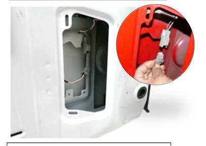
Step 4 Unplug 3<sup>rd</sup> brake light by firmly pressing down on the Mate-n-lock plug.
