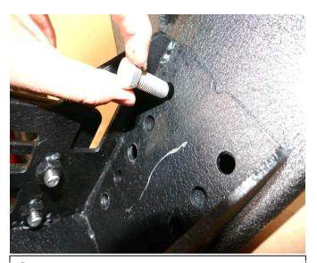
Step 4 Line up tire carrier arm holes to tire carrier. Place supplied M12 hex head bolts (C) onto tire carrier through tire carrier arm repeat same steps for remaining bolts.
