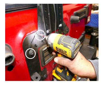
Step 2 Place brake light onto vehicle as shown. Place factory tire carrier hardware onto circled locations.
