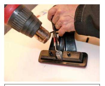
Step 6 Using a heat gun (or hair dryer if no heat gun is available) heat shrink tubes for a watertight connection.
