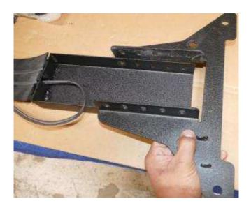
Step 9 Working on work bench. Install supplied brake light mounting bracket (L) onto supplied brake light (K) as shown. Line up brake light holes onto mounting bracket.
