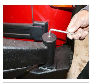
Step 5 Place the tire carrier cap onto tire carrier. Start supplied button head bolt into treaded hole in spindle. Tighten down with allen key.
