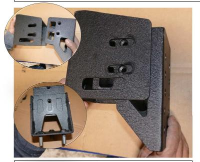
Step 1 Install supplied tire carrier mount (H) onto mounting bracket (I) as shown above. Line up mounting bracket holes to tire carrier side and lower center slots.
