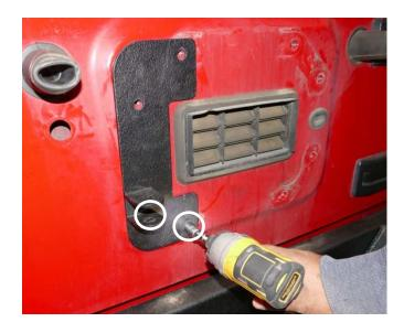
Step 1 Place supplied tailgate bracket (J) onto vehicle as shown. Place factory bolts onto the two locations circled above. Tighten down bolts.
