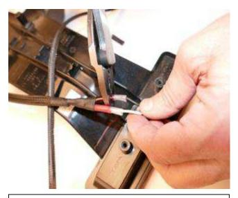
Step 5 Push the black connection onto the black cable. Crimp down to secure in place.
