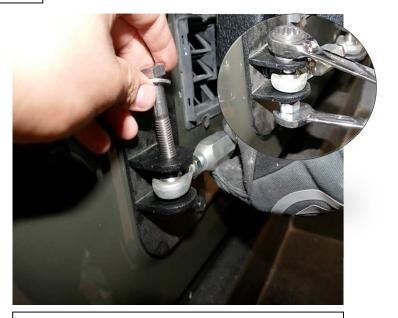
Step 2 With tire carrier closed install the other side of the turnbuckle onto tailgate bracket (J) by placing a supplied hex head bolt (Z) with supplied M12 washer (G) through the tabs in C plate and through the turn buckle. Place supplied M12 locknut at the end of bolt. Tighten down using a 19mm wrench and 18mm wrench.
