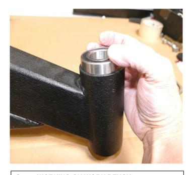
Step 3 **WORKING ON WORK BENCH**Place supplied sealed bearing (N) on the upper side of the tire carrier spindle hub. Carefully center bearing on the spindle hub and tap the bearing into position with a rubber mallet. Be careful to drive the seal
