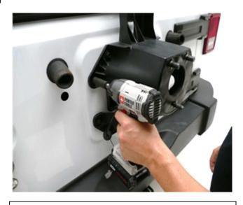
Step 6 Unbolt all 8 bolts (10mm socket) holding the OE tire carrier onto vehicle. Save hardware for reinstallation.
