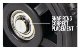
**3.** Pull up slightly on the wheel to ensure that the snap ring has seated in the groove. Repeat steps 2 and 3 on the remaining wheels.
