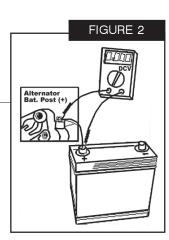
post (+) and the ground post (-). Voltage should be 13.8~14.5VDC. Readings above 15.5VDC indicate a defective alternator and readings below 12.7VDC indicate that the alternator is not functioning or cannot supply the current amperage needs of the vehicle at this engine speed.
