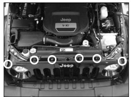
2. Remove 6 plastic retaining clips with flat head screw driver (locations shown above) by removing center rivet pin first.
