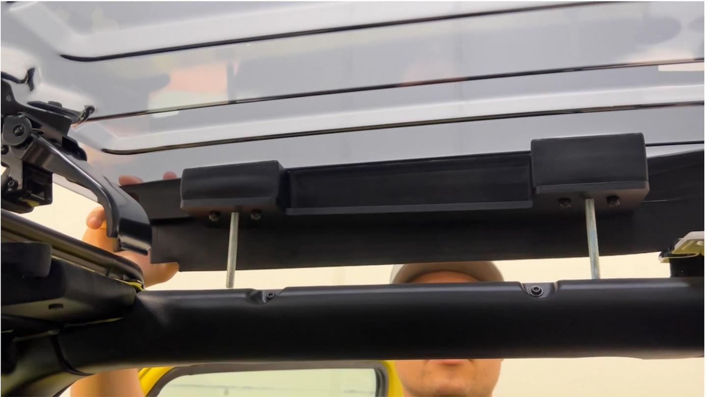
**Caution:** Leave the RED bolt covers on while installing the Sky View to avoid scratching paint while installing the Sky View lid.
