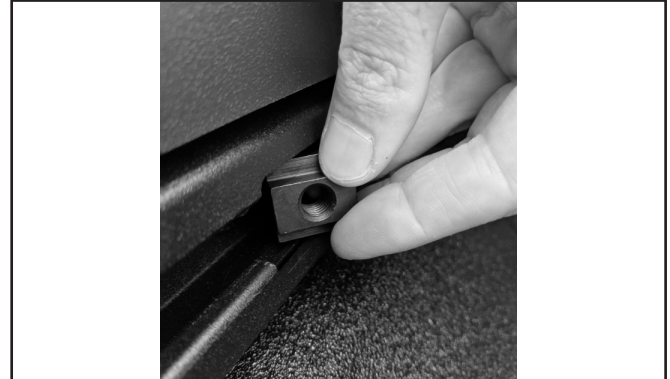
Figure 1: Inserting threaded nut plate into in-bed rail system
