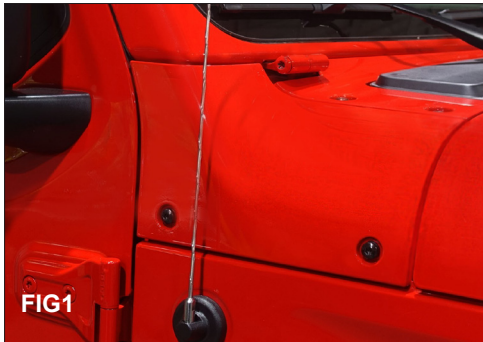
Put on safety glasses. (FIG 1) Using a 3/8" box wrench unscrew the antenna.
