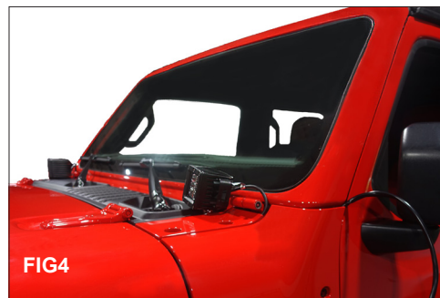
(FIG4) Run the wiring for the cube lights and light bar then re-install the Cowl. Using a T40 Torx bit socket loosely install the 2 top Cowl mounting screws. Repeat these steps for the driver side of the vehicle.
