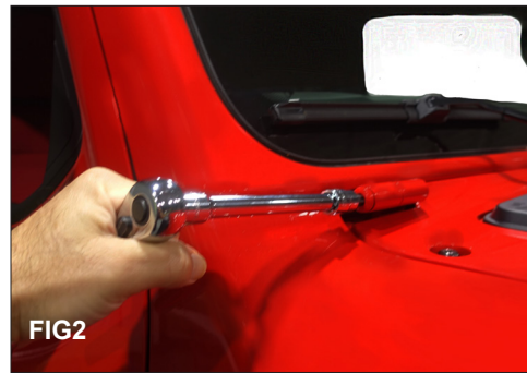
(FIG2) Using a T50 Torx bit socket remove the windshield hinge screw.
