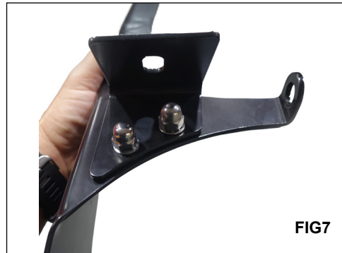
(FIG7) Align the bracket and Tighten all hardware to 6ft-lbs. Repeat for Driver side bracket.
