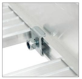
Install a reinforcing plate and nylock on the inside of the cargo basket as shown. Repeat on the remaining 3 holes and then tighten with a 17mm wrench.
