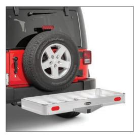
Install the assembled rack into the 2" receiver hitch on your vehicle and secure it with the supplied 5/8" hitch pin and cotter pin.
