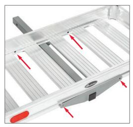
Place the Cargo basket onto the receiver tube assembly as shown with the reflectors facing the rear. Align the square holes in the reliever tube with the square holes in the cargo basket.
