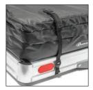
Take up slack in straps until the Cargo Storage Bag is securely attached to the cargo carrier.
