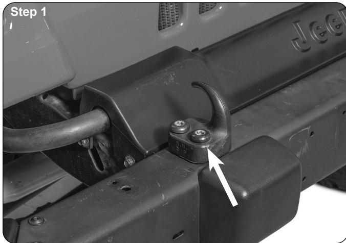
Put on safety glasses. Factory Bumper Removal: Using a T55 bit and socket remove the upper bumper bolts and/or tow hooks on both sides. (Step 1)
