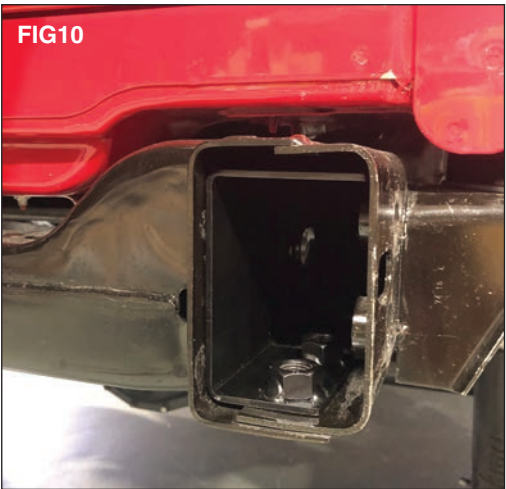
On the passenger side insert the supplied M14 nut plate into the frame rail. (FIG 10) Align the threaded holes in the nut plate with the holes in the frame on the bottom.
