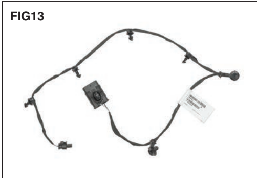
Bumper harness without backup sensors shown. (FIG 13) This bumper is not designed to work with backup sensors. Retain harness for use with optional license plate light (#12066 1100)
