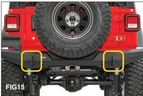
Loosely install the tow hooks through the bumper and into the bumper brackets with the supplied M10 allen head bolts and washers using a 6mm hex key. (FIG 15)
