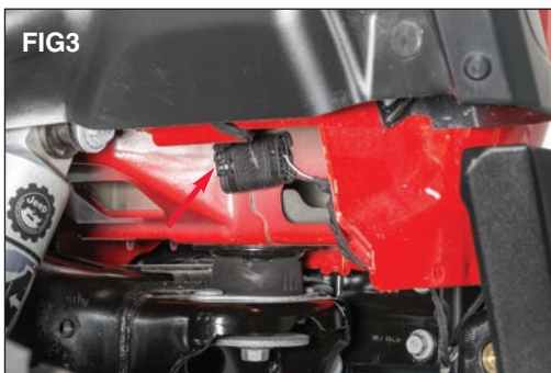
Disconnect the rear bumper harness by sliding the gray locking tab backwards and depressing the black tab. (FIG 3)
