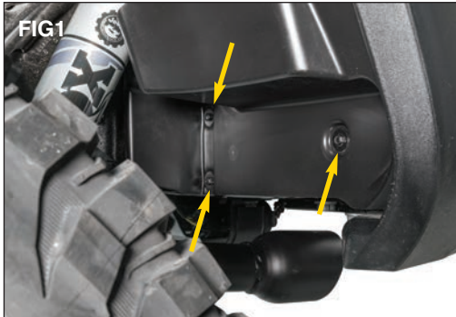
Put on safety glasses. Start by removing the factory splash guard. Remove the 6 screws holding the inner shields on, 3 on either side, using a 8mm socket. (FIG 1)
