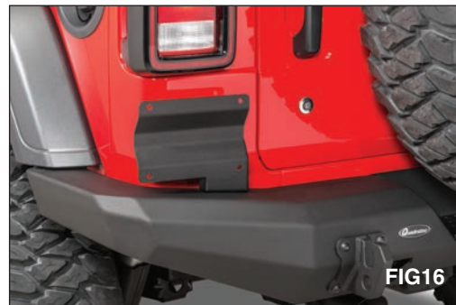
Once the bumper is aligned to your liking you may now tighten the M14 hardware to 105 ft/lbs and the M12 hardware to 65 ft/lbs.
