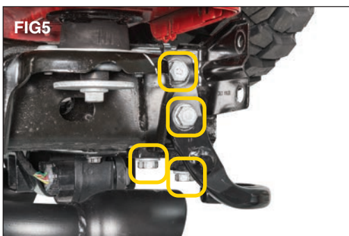
Remove the original tow hook if equipped using a 21mm socket. (FIG 5) Remove bumper bracket as well. There are 4 bolts total.
