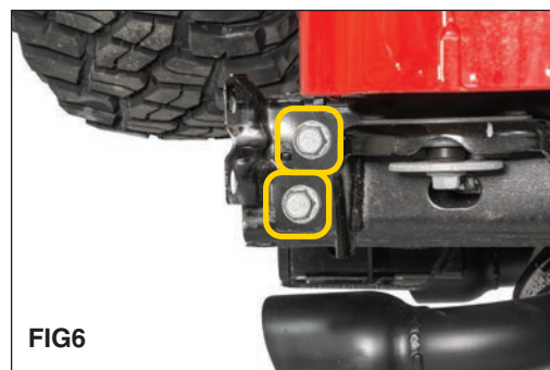
Remove the passenger side bumper bracket using a 21mm socket. (FIG 6)
