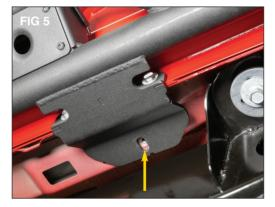
Locate the (3) vertical threaded holes behind the pinch weld. Align the holes in the brackets with these holes.(FIG 5) Install the 8mm hex bolts, lock washers, and washers using a 13mm socket. Repeat on other verticle holes. (FIG 6) Do not fully tighten at this time.
