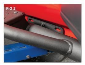
Starting at the front of the vehicle, position the mounting tabs of the side steps and align the holes with the factory pinch weld holes as shown. (FIG 2)
