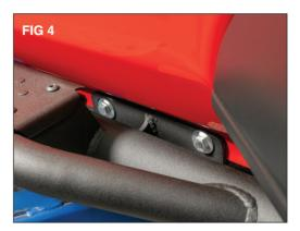
Do not fully tighten at this time. Repeat on the other side bracket holes. (FIG 4)
