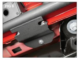
Then, holding the side step up on center with the pin weld holes fully tighten the 8mm pinch weld hardware. Once snug, you may now tighten the vertical 8mm bolts underneath. Repeat all steps on the opposite side. **Installation is complete.**
