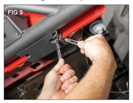
Install the 8mm hex head bolts through the pinch weld and the mounting brackets with washers on both sides and secure with a 8mm nylock nut using a 13mm hex wrench and a 13mm socket. (FIG 3)
