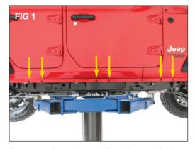
Put on safety glasses. Starting with the passenger side, locate the 6 holes along the factory pinch weld of your vehicle as shown. (FIG 1)
