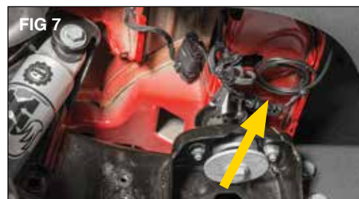
Loop the excess harness up out of the way and secure using the provided cable ties. (FIG 7)
