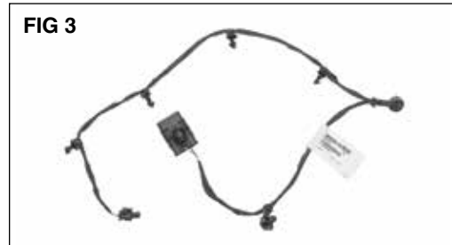
Disconnect all connections from the license plate light and backup sensors if present. (FIGs 2 & 3) New harness shown above (for reference) without backup sensors.
