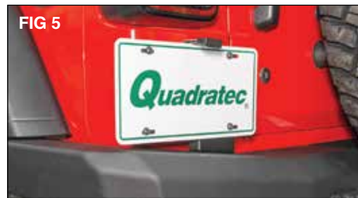
the way and secure using the provided cable ties. (FIG 4) Mount your license plate and the included light to the bumper's license plate bracket. (FIG 5)
