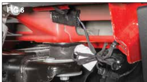
Route the light harness down towards the OEM bumper harness and connect it to the original license plate light plug until you hear a "click". (FIG 6)
