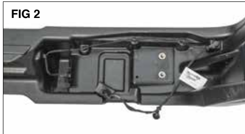
Put on safety glasses. Locate the bumper's wiring harness and remove all cable tie mounts using a clip/trim removal tool.
