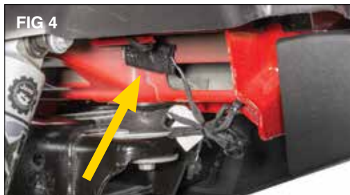
Reconnect the bumper harness to the vehicle until you hear a "click" and slide the gray locking tab to lock plug in place. Loop the excess harness up out of
