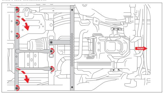
STEP 1: Put on safety glasses. Locate the Factory Transfer Casse cross brace. Remove the factory fasteners with 13 and 18mm sockets. The factory transfer case cross brace will not be reused, but be sure to keep all of the factory bolts for re-use.
