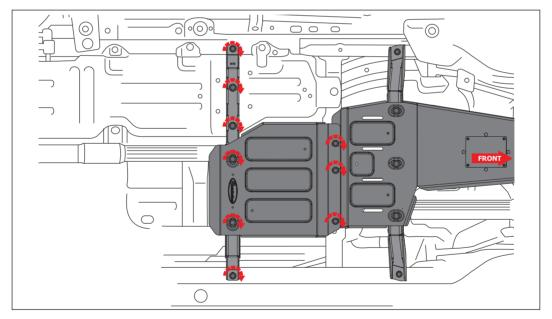
STEP 6: Next, make sure that all the skid plates align to your liking and then fully tighten all the fasteners with a 13, 17, & 18mm socket. Using a torque wrench tighten all M10 bolts to 36 ft lbs and all M12/factory fasteners to 48 ft lbs.
