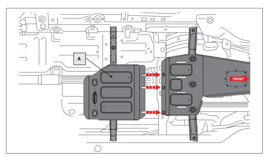
STEP 4: Slide the front of the Transfer Case Skid Plate (A) underneath the rear of the engine skid plate so that the slots line up with the bolts.
