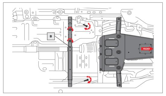
STEP 2: Using a 13 & 18mm socket, secure the new Cross Brace onto the frame using the factory transfer skid cross brace mounting locations and (4) factory fasteners. Snug but do not fully tighten the bolts at this time.
