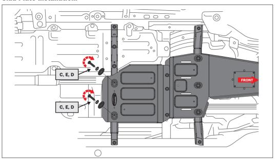
STEP 5: Install the (2) M10x30 bolts (C), lock washers (E) and flat washers (D) through the holes at the rear of the skid pate and thread them into the cross brace. Snug but do not fully tighten with a 17mm socket.
