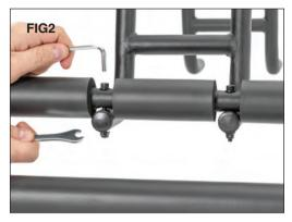
Secure the U bracket to the main rack with M6 x 60 cap screws (2), washers (4), and Nylock nuts (2). Tighten the bolts and nuts with the included M5 hex wrench and 10mm combination wrench. Repeat on opposite side.
