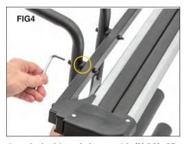
Attach the hinged clamp with (2) M6x65 cap screws, (4) washers, (2) plastic spacers, (2) nylocks. Place the plastic spacer between the outside of main frame and the hinged clamp. Tighten with the provided M5 hex and 10mm wrench. Repeat on opposite side.
