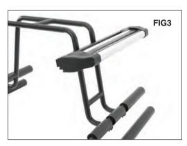
Position the hinged clamp over the upper holes in the main frame. Ensure the locking end of the clamp is facing the same direction as the open end of the u bracket.
