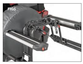
Adjust the cradles of your bike rack to fit the ski and snowboard rack. Place the rack into the cradles of the bike rack and secure it properly according to your bike rack instructions.
