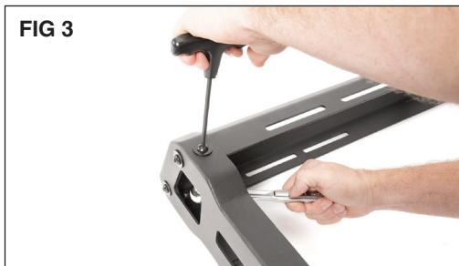
One corner one at a time, evenly tighten the top, bottom and side hardware using a 5mm hex key and 13mm box end wrench. (FIG 3)
