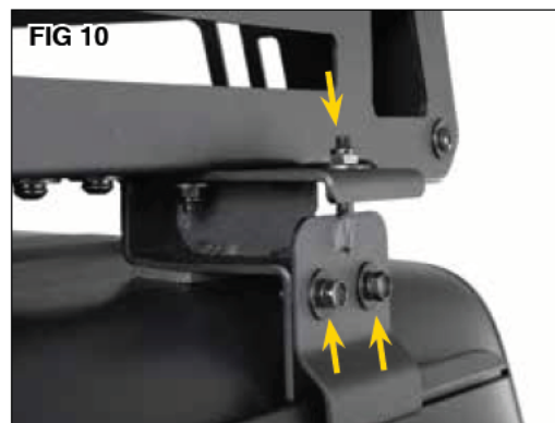
Now snug the top mounting stud using a 13mm deep socket. (FIG 10) Lastly tighten the side mounting bolts using a 13mm socket.
