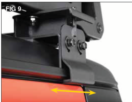
Once you have the rack in its desired location start by snugging the main brackets to the hard top. Bring the brackets clamp side mounting hardware just tight enough so it can still slide in the slots. (FIG 9)
