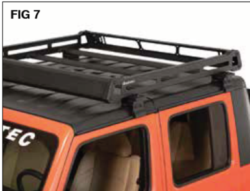
Once rack is assembled per its directions, with help from an assistant lift it up onto the brackets carefully aligning all the mounting slots. (FIG 7)
