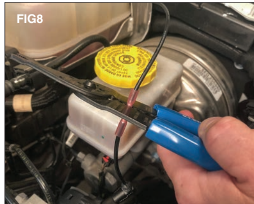
Connect the black wire from your J-Series light bar to the barrel connector and then used a heat gun to shrink the connector which provides a weather tight seal. (FIG 8)
