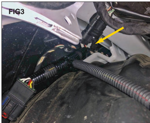
Plug in the new Tee harness to each side of the OEM harness until you hear a click and then push the red and gray locking tabs to lock the connections. (FIG 3)
