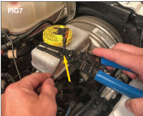
On J-Series light bars cut the fused end off and strip the end of the wire. (FIG 7)
