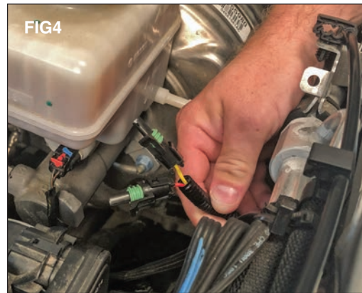
Route the two weather tight connectors up to the engine bay for easy access. (FIG 4)
