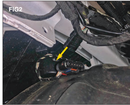
Slide the red locking tab backwards and disconnect the plug. (FIG 2)
