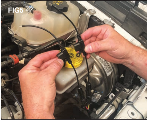
Connect the fused pigtail to the desired connector. (FIG 5) The yellow wire is for running lamps such as J-Series light bars. The red wire is for vehicles with daytime running lamps and will have 12 volts when the engine is running.
