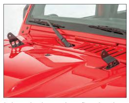
bolts and nylon washers. Snug but do not fully tighten the bolts using a T40 Torx bit or key.
