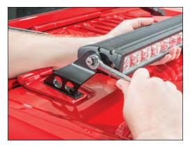
While supporting the light bar pass the stud through the hole on the Passenger hood bracket and secure it with a washer, split washer, and nut. Tighten using a 13mm wrench.
