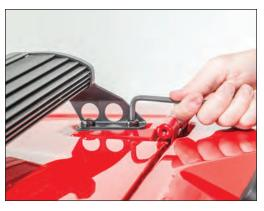
Fully tighten the hood fasteners at this point with a T40 key.
