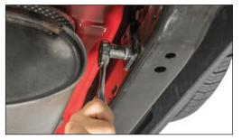
Proceed to Remove the bolts with a ratchet and a 16mm socket. Three mounting holes are provided for various
