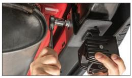
Place the light mount over the factory bumper bracket and reinstall the factory bolts with a 16mm socket. The light mounts have slotted mounting holes to
