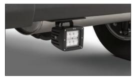
allow for vertical adjustment. If you do not have the factory bumper or mounting brackets you can use a M10 x 1.25 x 35mm bolt. Repeat for opposite side.
