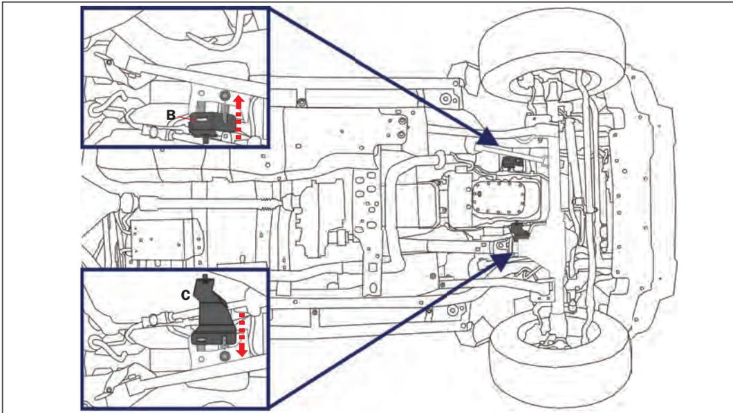
**STEP 3:** Slide the Left (C) and Right (B) Mounting Brackets into place so that the slots slide behind the front bolts & washers.
