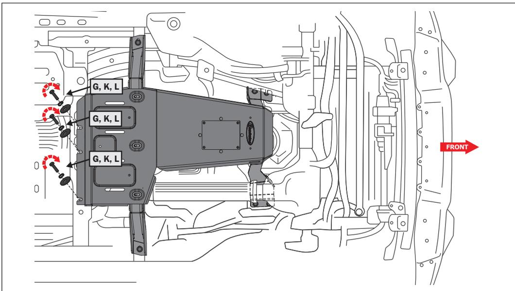
**STEP 8:** Install the (3) M12x40 bolts (G), lock washers (K), and M12 flat washers (L) into the remaining rear holes of the skid plate. Snug but do not tighten.
