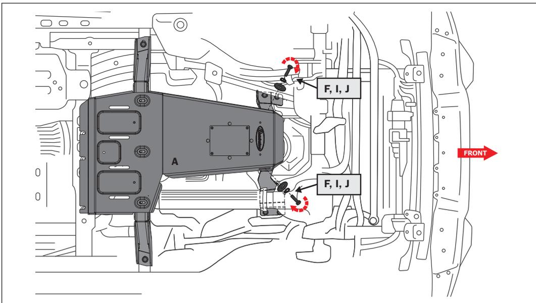
**STEP 6:** With help from a friend, lift the skid plate (A) into place and attach the front of the skid plate to the mounting brackets (B&C) with (2) M10x30 bolts (F), lock washers (I) & flat washers (J). Snug the bolts with a 17mm socket, not fully tight.
