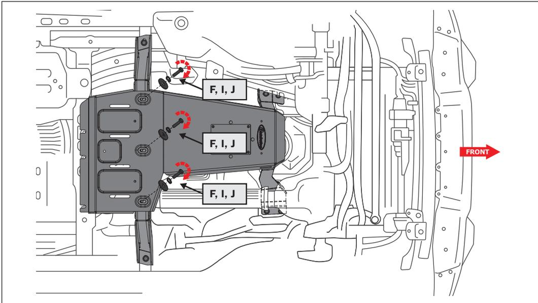
**STEP 7:** Install (3) M10x30 bolts (F) with lock washer (I), and flat washer (J) into the front 3 holes in the skid plate and thread them into the cross brace. Snug but do not tighten.
