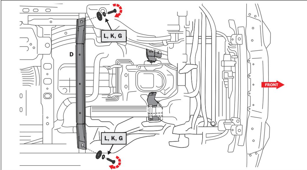
**STEP 5:** Install the Cross Brace (D) into existing holes in vehicle frame with (2) M12 bolts (G), lock washers (K), and flat washers (L). Snug but do not tighten the bolts with a 19mm socket to allow for alignment before final tightening.
