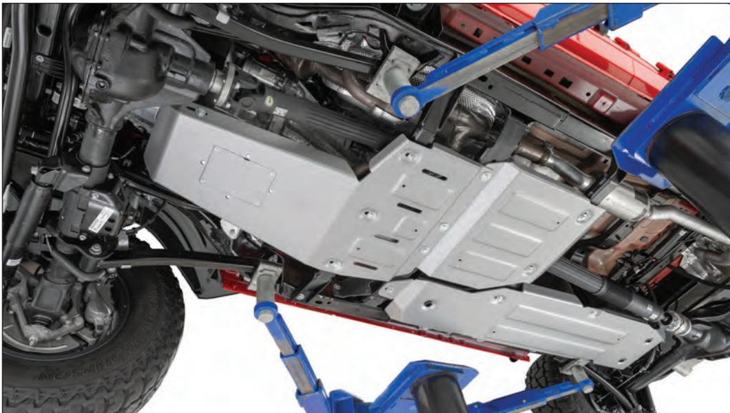
Installation is complete. This also shows the Transfer Case Skid Plate and the Fuel Tank Skid Plate (sold separately).
