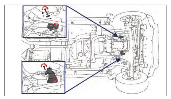
**STEP 4:** Install the other (2) M10x20 Bolts (E), lock washers (I), and flat washers (J) into the rear slot of the mounting brackets and hand tighten the bolts into the nut plates (H). Snug but do not fully tighten all the M10x20 bolts with a 17mm socket.
