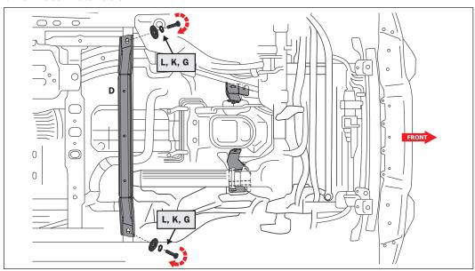
**STEP 5:** Install the Cross Brace (D) into existing holes in vehicle frame with (2) M12 bolts (G), lock washers (K), and flat washers (L). Snug but do not tighten the bolts with a 19mm socket to allow for alignment before final tightening.
