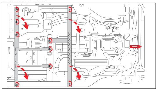
**STEP 1:** Put on safety glasses. Locate the Factory Transmission Cross brace (automatic only) and the Factory Transfer case skid plate. Remove the factory fasteners with 13 and 18mm sockets. The cross brace & transfer case skids will not be reused, but be sure to keep all of the factory bolts for re-use.
