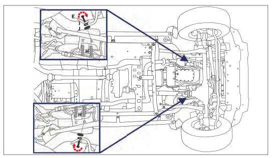
**STEP 2:** Locate the engine frame ears where the engine attaches to the frame. Slide the (4) M10 Nut Plates (H) inside the frame ears so that the threaded hole aligns with the holes in the frame. Finger tighten (2) M10x20 bolts (E), M10 lock washers (I), and M10 flat washers (J) into the front hole on either side.
