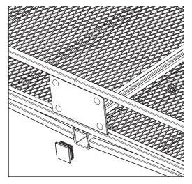
Insert the plastic plug into the end of the tube. At this time, tighten all M10 and M12 fasteners.
