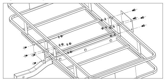
Place the 2 connecting plates on either side of the rack. Secure the plates in
