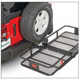
Install the rack into your 2" receiver hitch and secure with the supplied 5/8" receiver pin and cotter pin.
